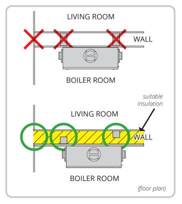
Figure 12 Recommended wall construction
