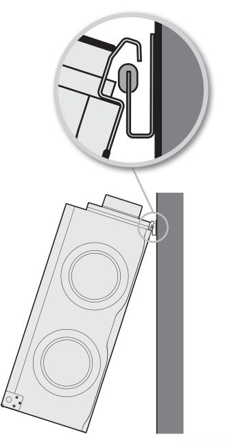
Figure 15 Fitting the wall bracket
