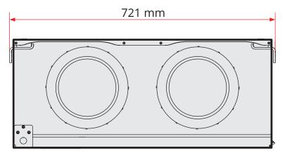
Figure 9 Holes, side mounting
