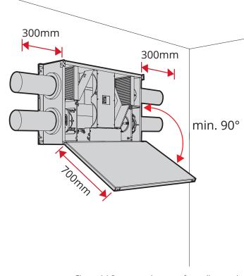
Figure 14 Space requirements for wall mounting
