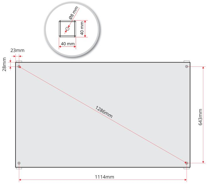
Figure 5 Holes, top mounting
