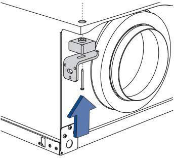
Figure 6 Mounting bracket, top mounting
