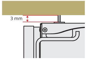
Figure 7 Gap to mounting surface
