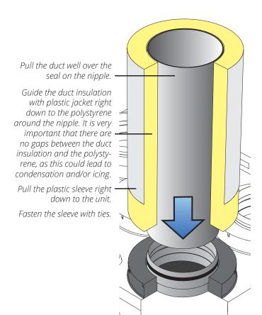
Figure 20 Duct connection
